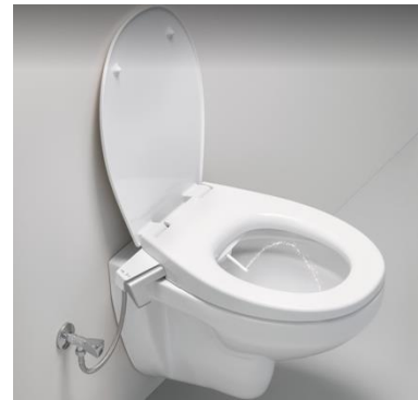
Figure 7. Example of a bidet/douche toilet seat fixed to a toilet pan, with a below-the-rim fixture. This does not have a 25mm RAG. This may require a high hazard backflow prevention device, depending on its Watermark certification.
