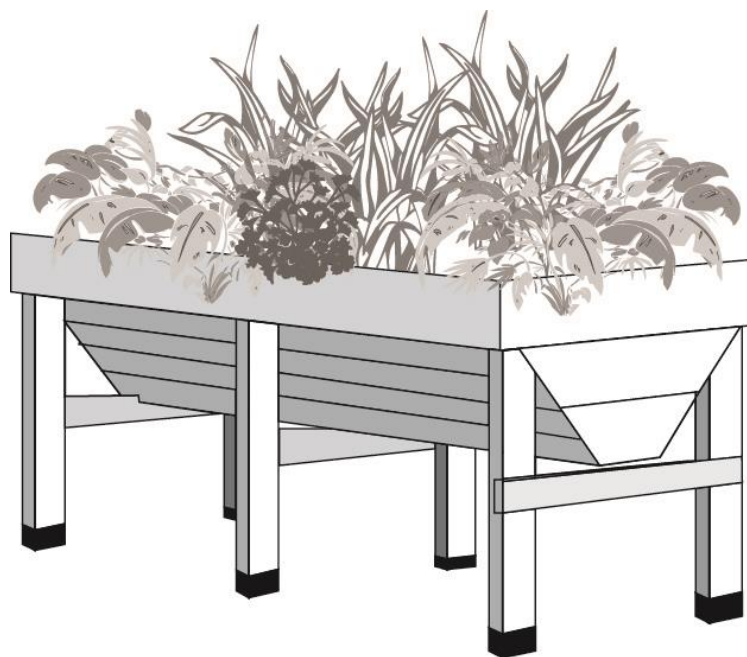
Figure 2. Example of a table planter providing under table access for seated gardening in a chair or wheelchair.
