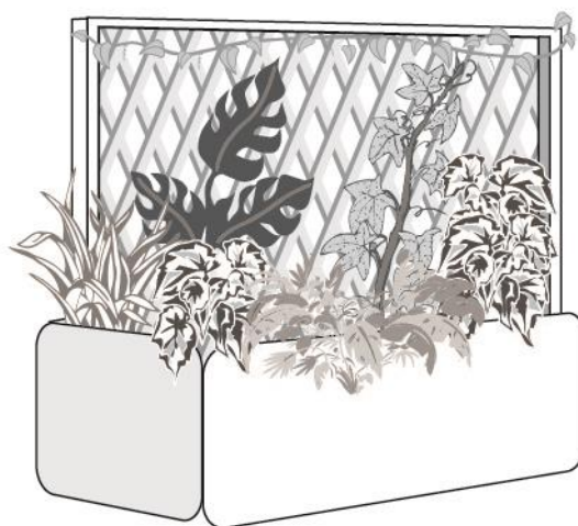
Figure 3. A typical Green façade arrangement. Shows the pot containing growing medium plants which will grow up in a supportive frame.
