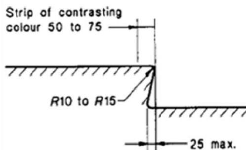
Figure 3. Recommended nosing design (source: Standards Australia, 1992a)
