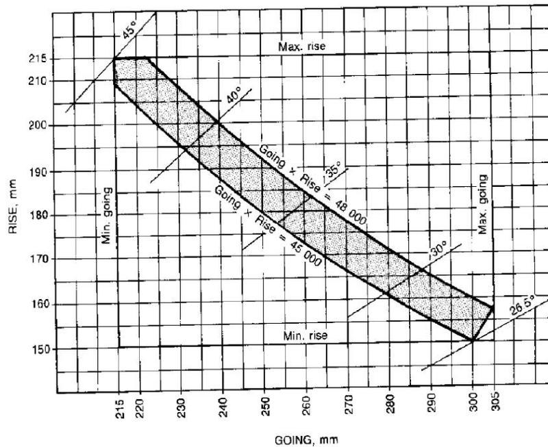
Figure 2. Suitable stair dimensions (source: Standards Australia, 1992a)
